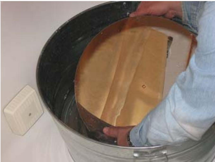
After thoroughly rinsing the mirror with warm tap water, it is time for hopefully, the final rinse.
