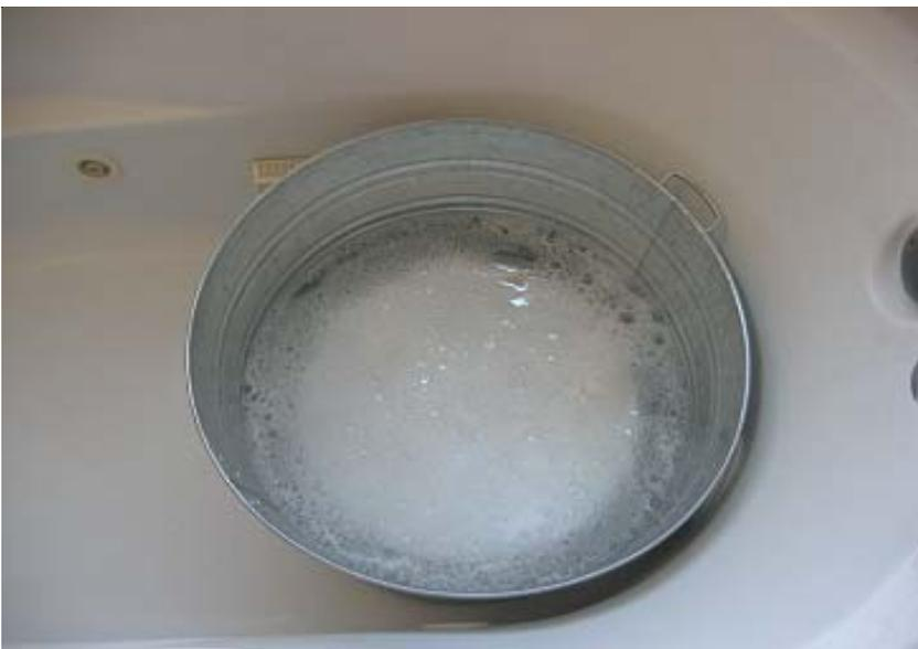
First, carefully remove the mirror from the telescope. Then place the mirror, mirror side up, in the tub. Next fill the tub with warm water to a point where it just covers the mirror. Add a few drops of mild dish washing liquid soap and then add enough additional water to properly mix the soap. I used my removable shower head. Then go do something else and let the mirror soak for an hour or two. This should allow the soap and water enough time to dissolve any oils on the mirror.
