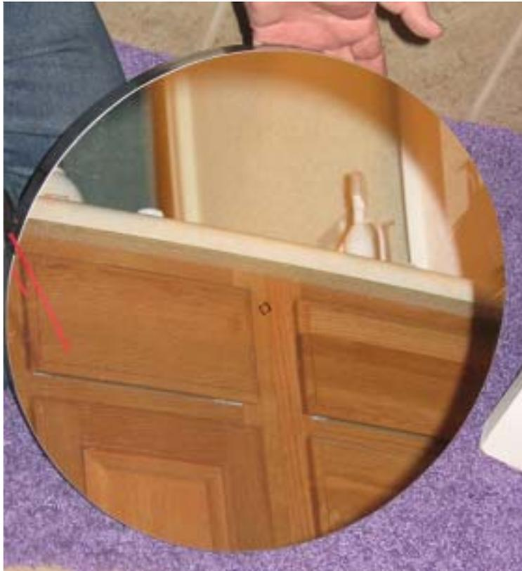
Chase the remainder of the water from the mirror surface with a can of compressed air, sometimes called Dust Off. Lowes again had this as did Best Buy. If after chasing all the water droplets off the mirror you see dried water spots on the mirror Rinse it again. This time use a mixture of 75% distilled water and 25% alcohol (denatured alcohol) Tequila is not an acceptable substitute. Then again chase the droplets off the mirror surface.
