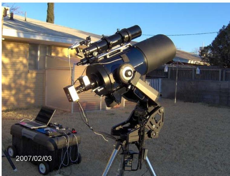
After a few sessions of wide-field photography, I decided to try attaching the camera in place of the telescope eyepiece, which would let me take less panoramic shots of smaller objects. I found that alignment was much more critical since longer exposures were needed to capture faint images, and alignment errors were more noticeable at higher magnifications.
