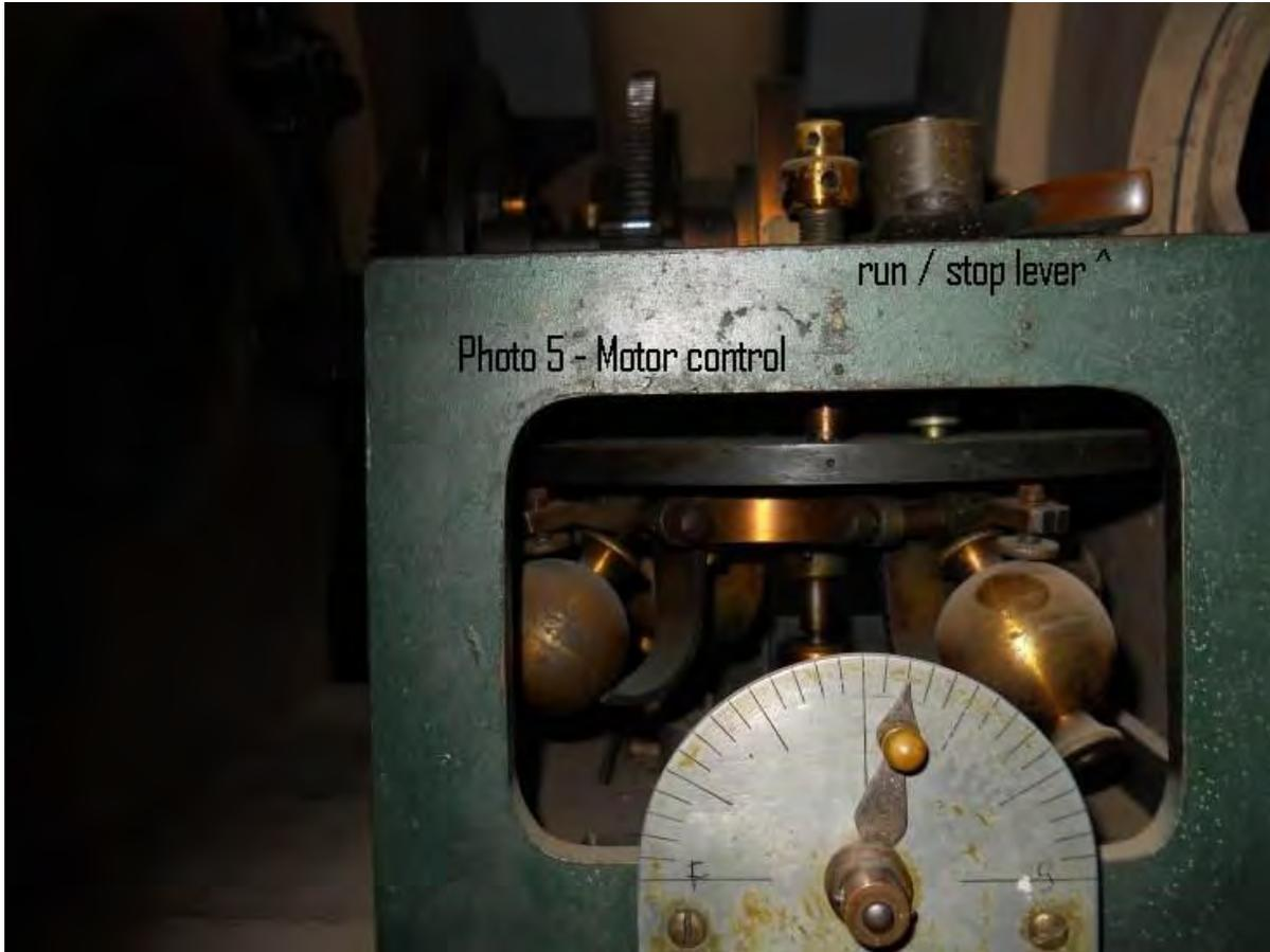
Move the lever on the top of the green housing to the left to start the gravity motor. The telescope should now be moving in right ascension compensating for the earth's rotation. The pointer above the scale marked F / S (fast / slow) controls tracking speed by adjusting the fly-ball governor. It needs to be adjusted for the type of target being tracked such as star, planet, or moon. It will require trial and error to find the right speed.
