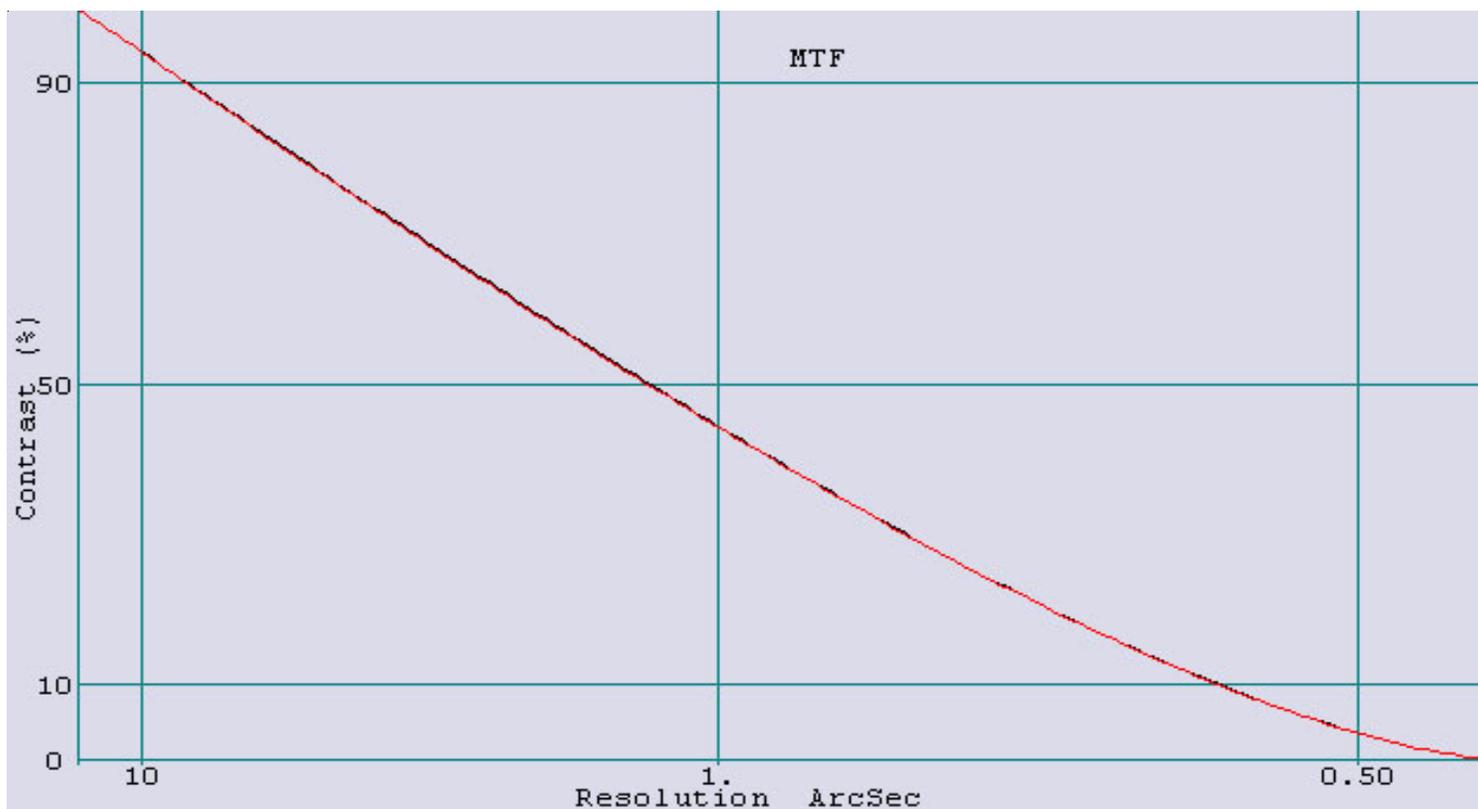
The horizontal scale of the graph expresses resolution or spatial frequency. This is often shown in lines per millimeter but I've substituted angular spacing in arc/sec to make the result more meaningful. The vertical scale represents contrast. The curve shown is how much contrast is lost from reality at different spatial frequencies.
