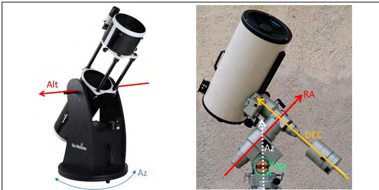
**Figure 4:** The two major types of telescope mounts. The left is an Altitude-Azimuth mount comprising a Dobsonian telescope. On the right is a German Equatorial mount that incorporates the ability to adjust the altitude and azimuth of the equatorial head (denoted by the Az and Alt labels).
