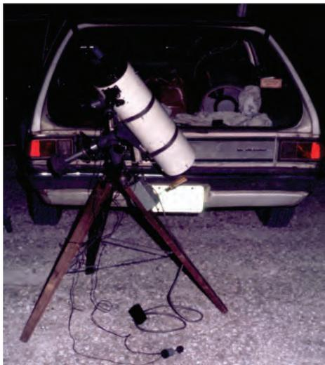
*The six-inch f/4.5 Newtonian that provided a platform for these photos of Comet West. The telescope has electric slow motions on both axes. The telescope is powered from the car with a special outlet just inside the back of the car. The outlet is wired back to the fuse panel.*
