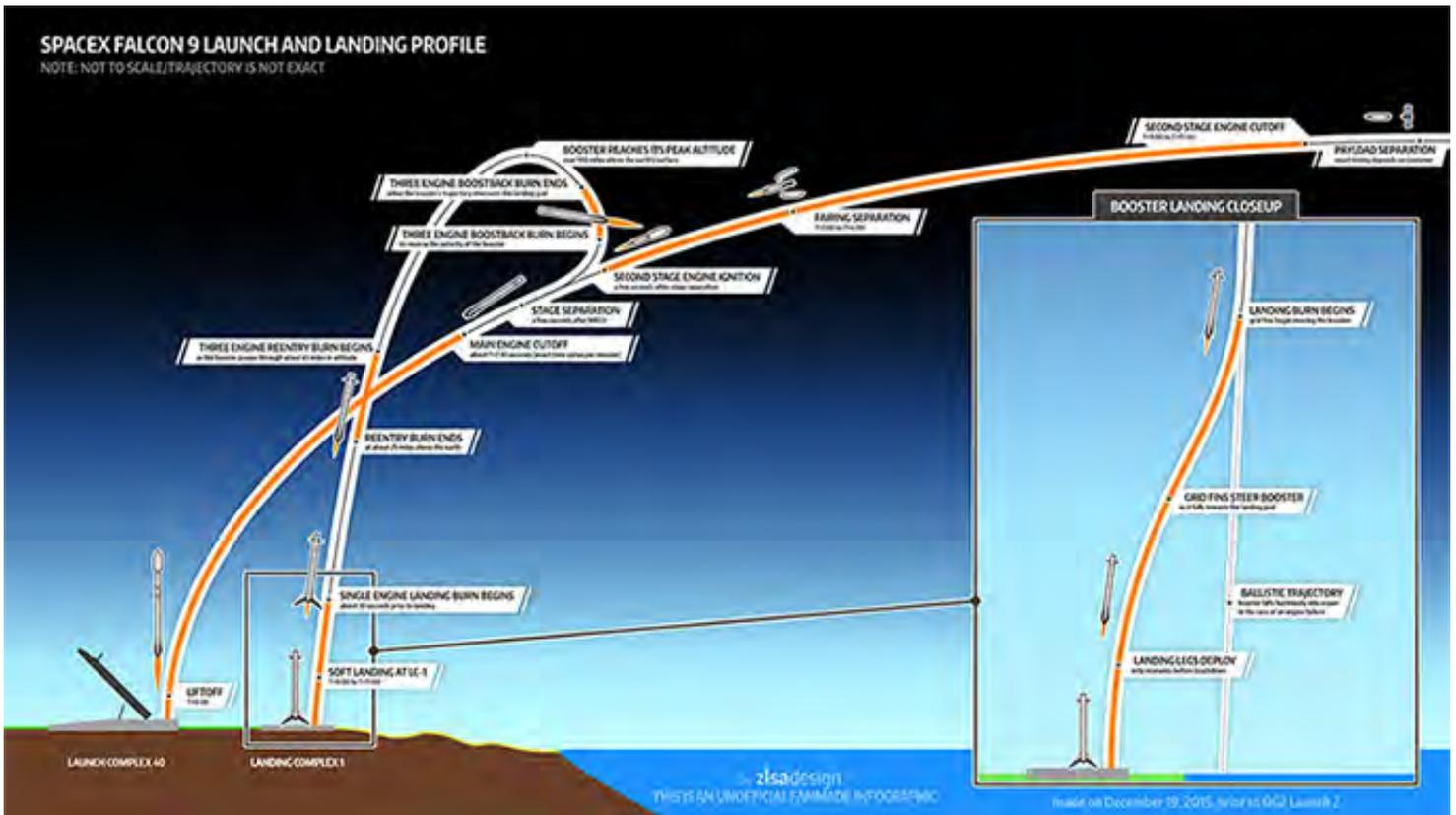
**Figure 2:** The diagram of the flight profile of the Falcon 9 with a landing back at the Kennedy Space Center shows that if the payload is not too heavy, the booster can be flown back to the launch area and land on solid ground. The engine burn to slow the booster down uses three of the seven Merlin engines. Landing back at Kennedy saves time and costs since the drone ship does not have to be taken out to the landing zone and then returned.
