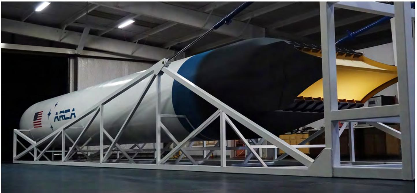
*Figure 3: Here the Haas 2CA rocket is sitting on a cradle in a hanger at the Las Cruces International Airport. The initial design is a single-stage-to-orbit for small payloads. Future designs will include a second stage to triple the payload that be placed in low Earth orbit.*
