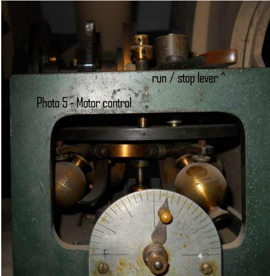
Move the lever on the top of the green housing to the left to start the gravity motor. The telescope should now be moving in right ascension compensating for the earth's rotation. The pointer above the scale marked F / S (fast / slow) controls tracking speed by adjusting the fly-ball governor. It needs to be adjusted for the type of target being tracked such as star, planet, or moon. It will require trial and error to find the right speed.
