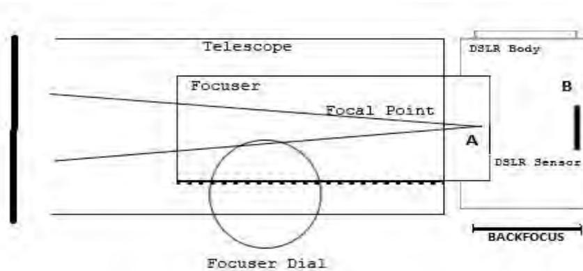
It required some research to determine the back-focus distance for the Canon EOS T1i. It required determining the distance from the image sensor to the middle of the bayonet flange. Also the T-ring adapter dimension has to be considered. It was determined that 44mm were required from the bayonet flange to the image sensor and another 12 mm was required for the T-ring adapter. All together about 2.25 inches of back-focus was necessary.
