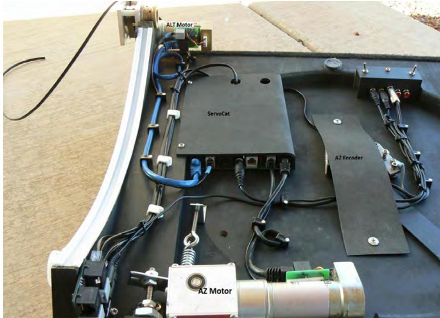
The system can track an object with good consistency depending on location in the sky. It clearly is not a match for an equatorial mount but I have tracked an object over one hour. Guiding is supported by the **ServoCat** but there is no practical way to mount a guide scope on the 18" UC. A Telrad is used for locating object areas. The tradeoff is tremendous light gathering but only for shorter intervals.
