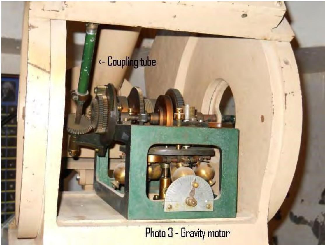
Sliding the green coupling tube upward engages its bevel gear with the mating gear and couples the gravity motor to the telescope. Look at the worm wheel sector. If it is not at the beginning of its travel, it should be rewound. See the description for this below. After the worm wheel sector is set to the beginning of its travel, slide the green coupling tube upward and tighten its clamp.
