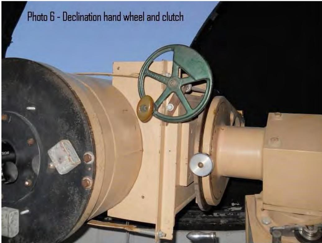
Photo 6 - Declination hand wheel and clutch
