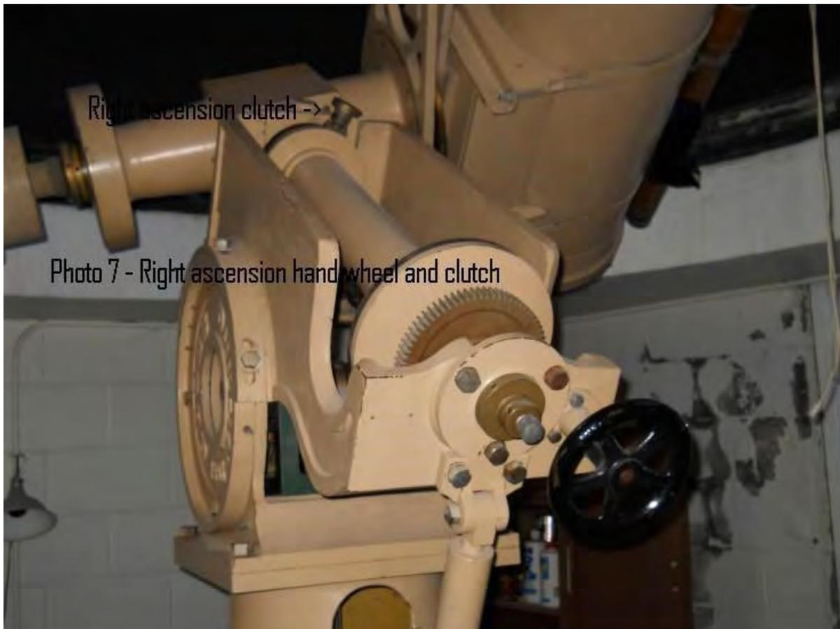
Photo 7 - Right ascension hand wheel and clutch
