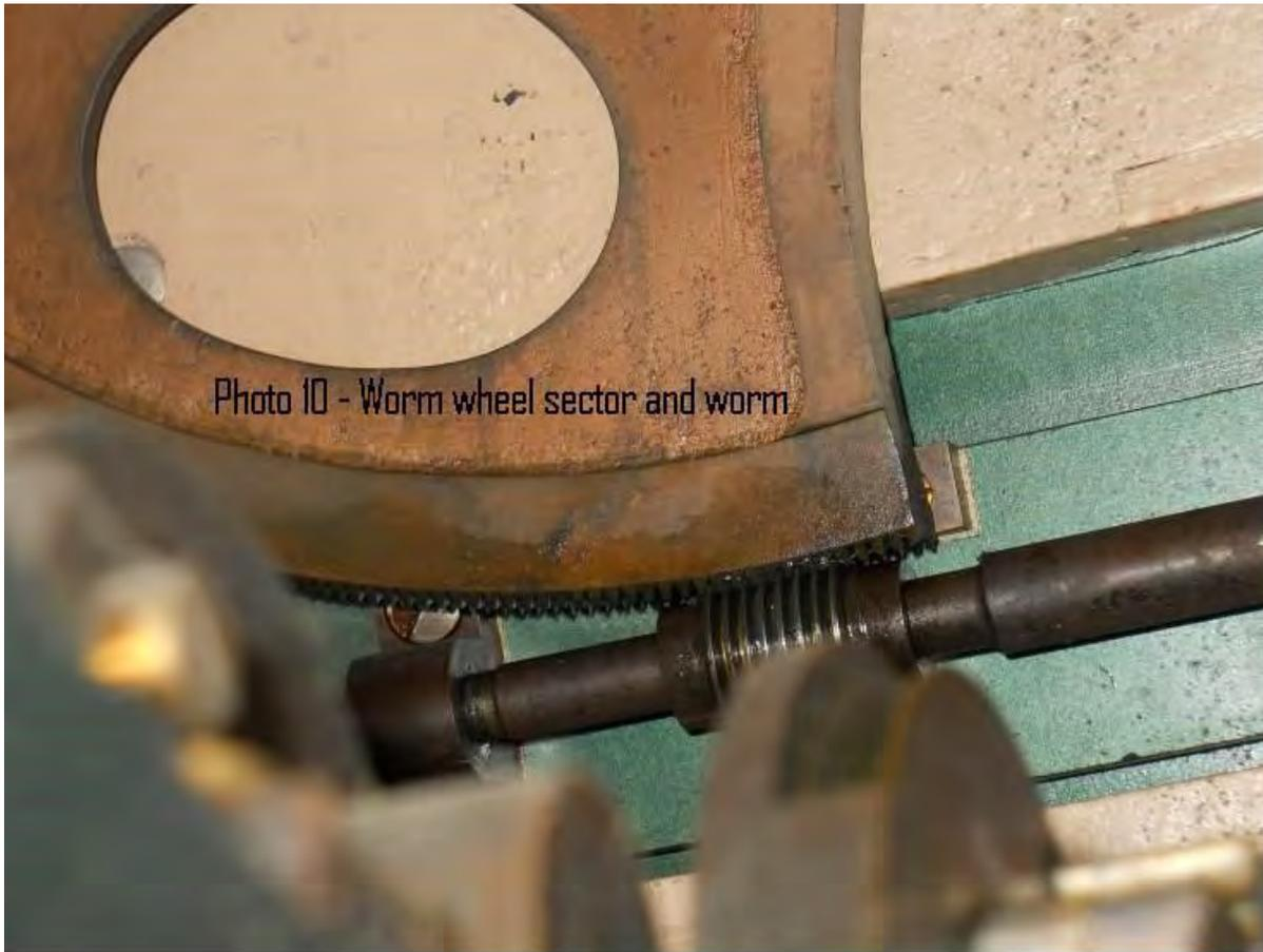
Turning the crank moves the right ascension worm wheel sector back to its starting point. The telescope will have to be moved back on target after moving the worm wheel sector. Reengage the motor by raising the green coupling tube until the bevel gears engage and tighten its clamp. The only thing to remember in moving the telescope is to keep the optical tube pointing above horizontal. Moving downward past horizontal may let internal mirrors move out of place.
