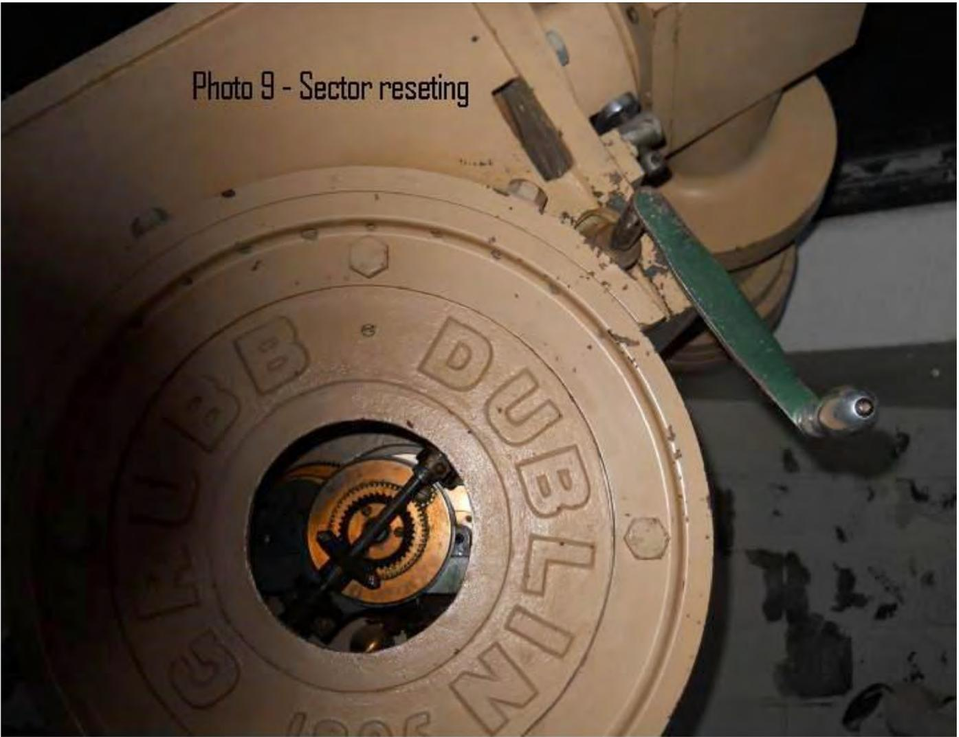
If the worm wheel sector has reached its end of travel, disengage the motor by loosening the clamp on the green coupling tube. Then remove the crank from its square pin, placing it on the square pin on the opposite side as shown above. Turn the crank clockwise while facing it. This will turn the worm and move the worm wheel sector back to its starting point.
