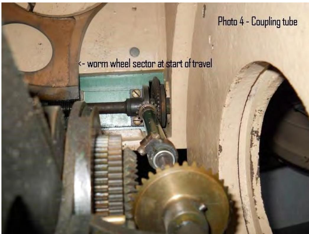
The photo shows the green coupling tube from inside the frame. The bevel gear pair at the bottom connects the gravity motor shaft from the fly-ball governor to the green coupling tube. The green coupling tube has another bevel gear at the top which engages with one above it on the worm shaft. Slide the tube upward until the bevel gears engage and tighten the clamp to keep it in place. The gravity motor is then coupled to the worm wheel sector which moves the telescope in right ascension.
